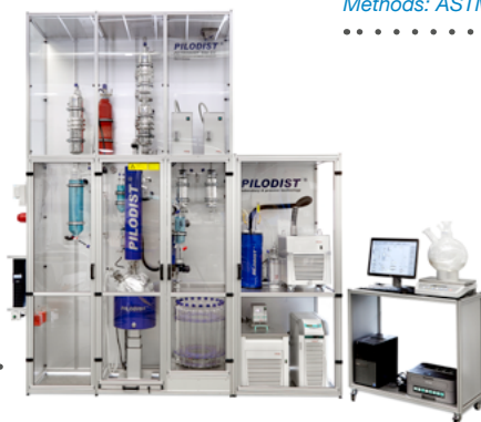
PETRODIST 350CC Fully Automatic Methods: ASTM D1160
