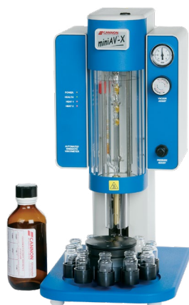
CANNON miniAV-X – A fully automated, single-bath, benchtop viscometer with a 10-position sample handler for unattended D445 processing
