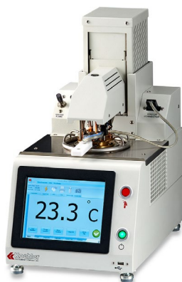
Automatic Pensky-Martens Closed Cup Flash Point Tester
