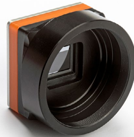
Dione 640 CAM Series Uncooled 12 µm pitch microbolometer detector with a 640x480 resolution and NETD of less than 60 mK
