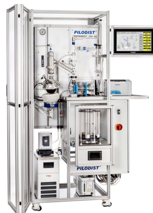
PETRODIST 350CC – Fully Automatic Methods: ASTM D1160
