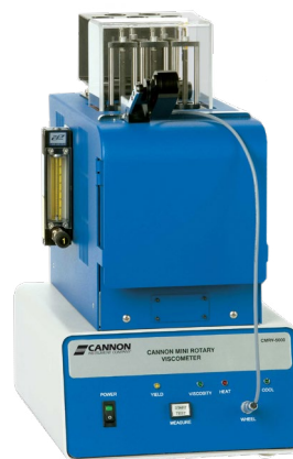
CMRV-5000 – The semi-automated CMRV-5000 is a compact and completely self-contained mini-rotary viscometer for measuring low temperature pumping viscosity from -5^{\circ}\text{C} to -40^{\circ}\text{C}
