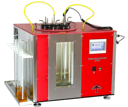
TFAB Tannas Foam Air Bath Methods: ASTM D892, D6082, D1881, D7840
