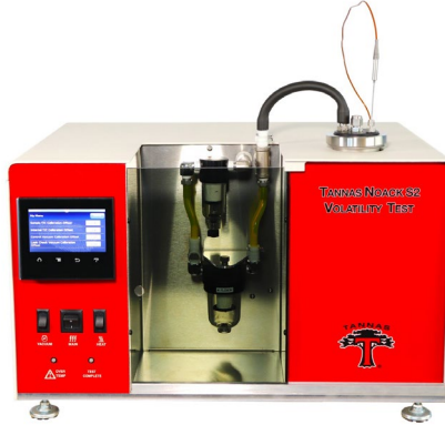
Noack S2 Volatility Test Methods: ASTM D5800, CEC L-40-93
